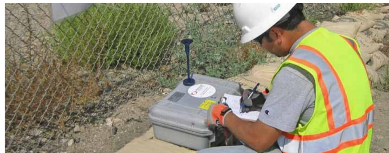
TECHNICIAN PERFORMING ROUTINE INSPECTION AT ONE OF SEVEN AIR MONITORING STATIONS
